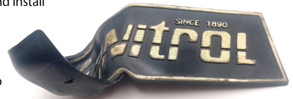
Melted sign off of overheating HVAC unit.
